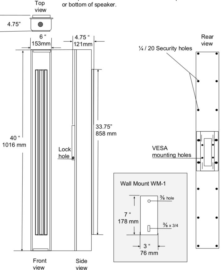
Mounting plate may be affixed to any of the sets of security holes in the rear of the cabinet to meet differing installation requirements.
